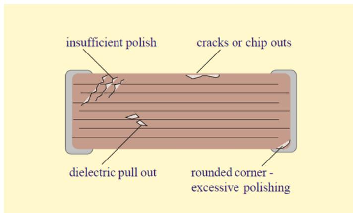
Figure 30. Sample preparation defects
