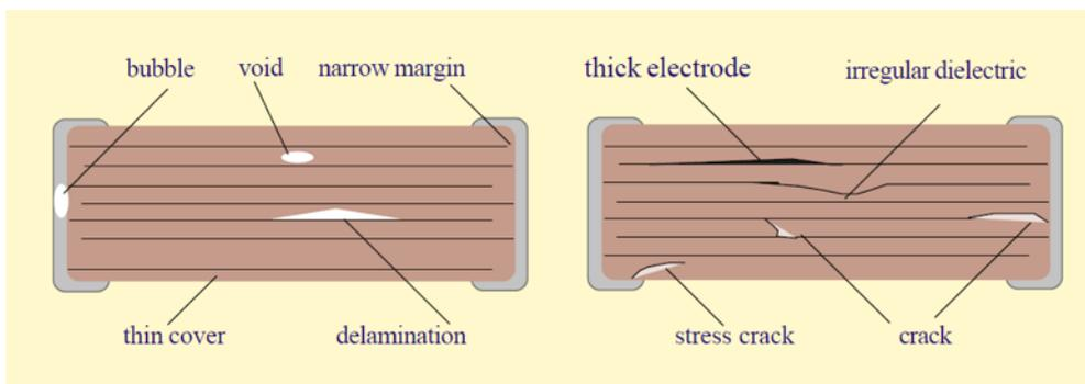
Figure 29. Microstructure Defects
