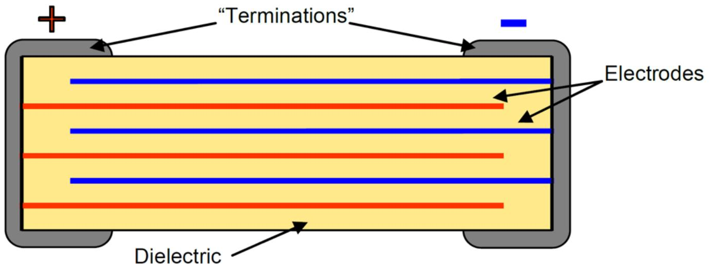
Figure 7: A Diagram of an MLCC
