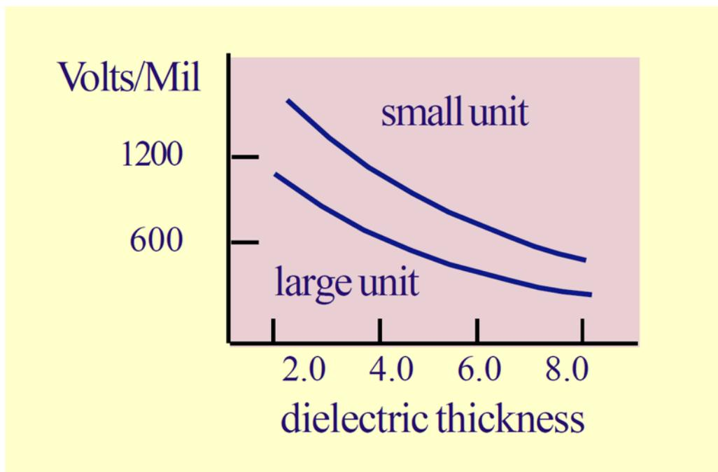
Figure 12: Dielectric Strength vs Dielectric Thickness
