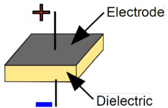
Figure 6: A Diagram of a Single-Layer Capacitor
