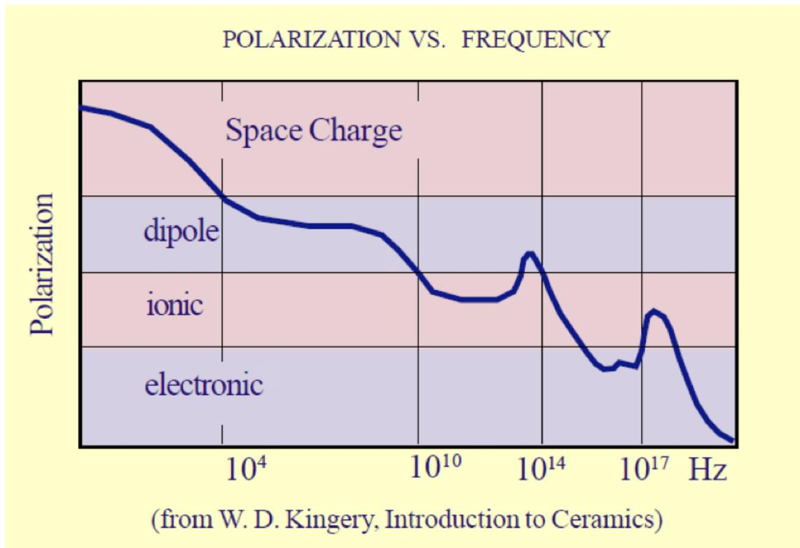
Figure 9: The Effect of Frequency on Polarization Mechanisms
