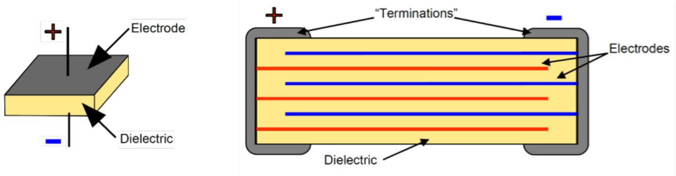
Figure 2. Single Layer Capacitor (Left) Versus a Multilayer Capacitor (Right)
