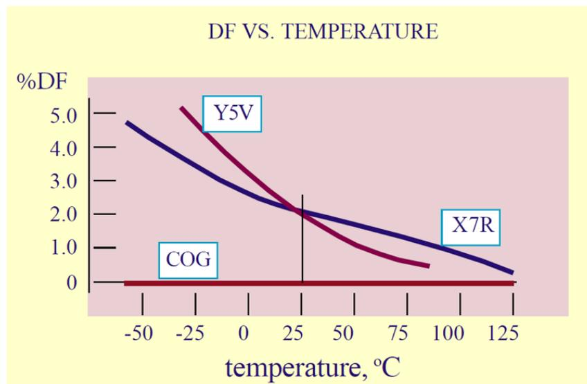
Figure 22. Dielectric Dissipation Factor Curves With Temperature
