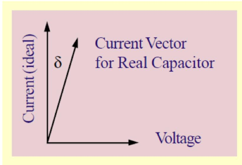
Figure 31. Loss Tangent in a Real-World Capacitor
