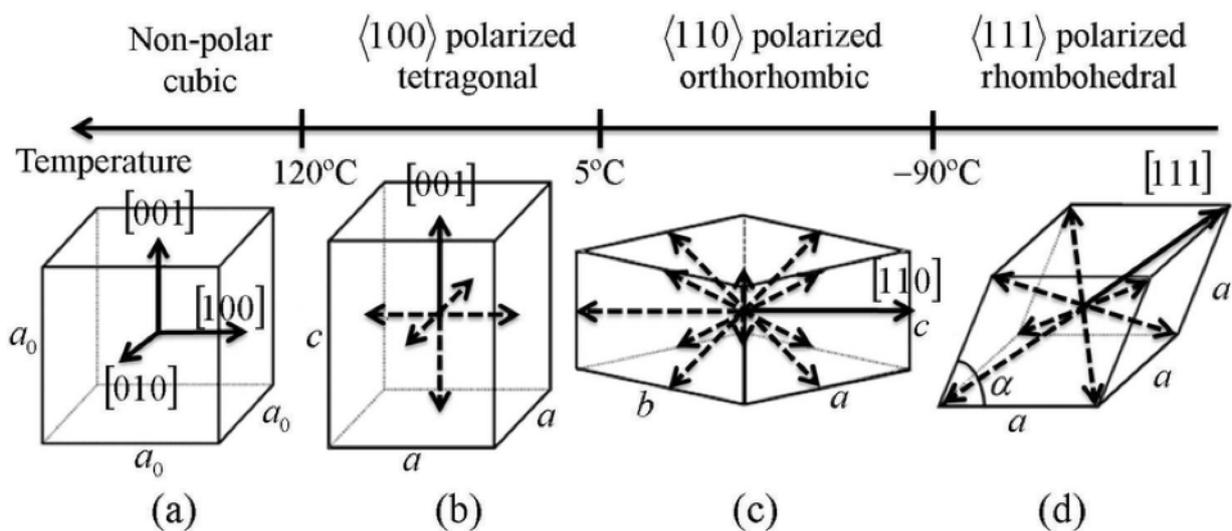
Figure 17. Phase Transformations of BaTiO<sub>3</sub> (source: University of Oxford)
