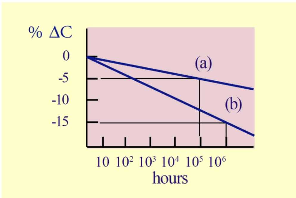
Figure 13: Ferroelectric Aging Shown as Percent Change in Capacitance (% $\Delta C$ ) Over Time
