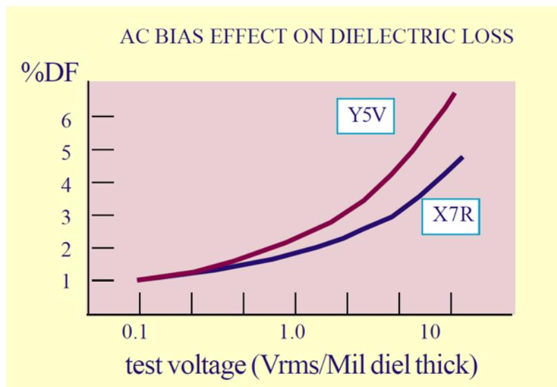
Figure 25. AC Bias Effect on Dielectric Loss
